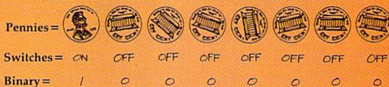
Figure 4: A Byte Holding The Screen Code For Letter A (65)
